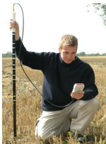
Fig. 3 TDR probe capable of reading soil moisture at multiple depths..
