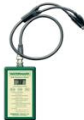
Fig. 4 Handheld device for taking readings from Watermark Soil moisture probes.
