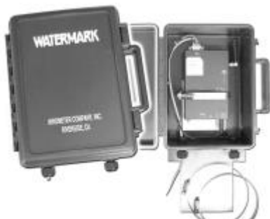
Fig. 5. Station for sending soil moisture data via a cell phone link.
