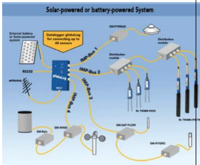
Fig. 6. Diagram of systems available for automatically reading and recording data from multiple TDR probes.
